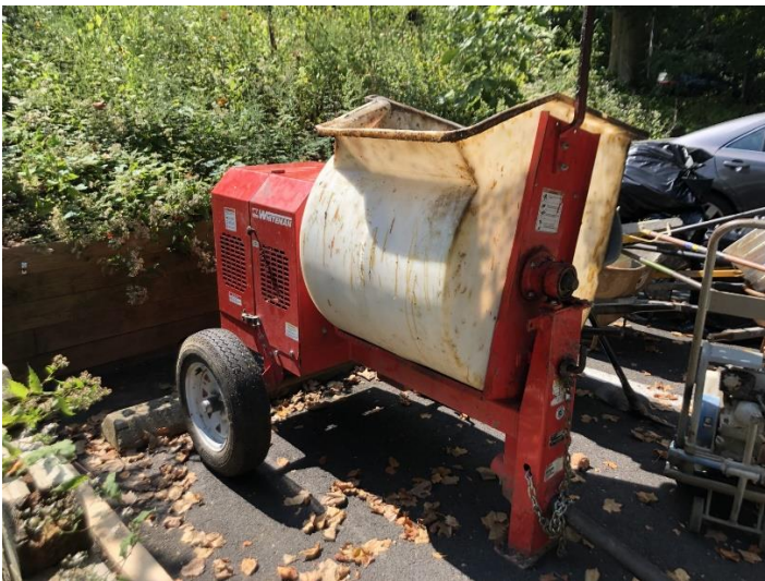
The plaster/mortar mixer used for the Porous Pave
